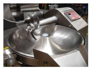
Figure 2: Bowl chopper. Photo: Courtesy of Union Food Machinery Ltd. <a href="www.ufm-ltd.co.uk">www.ufm-ltd.co.uk</a>.
